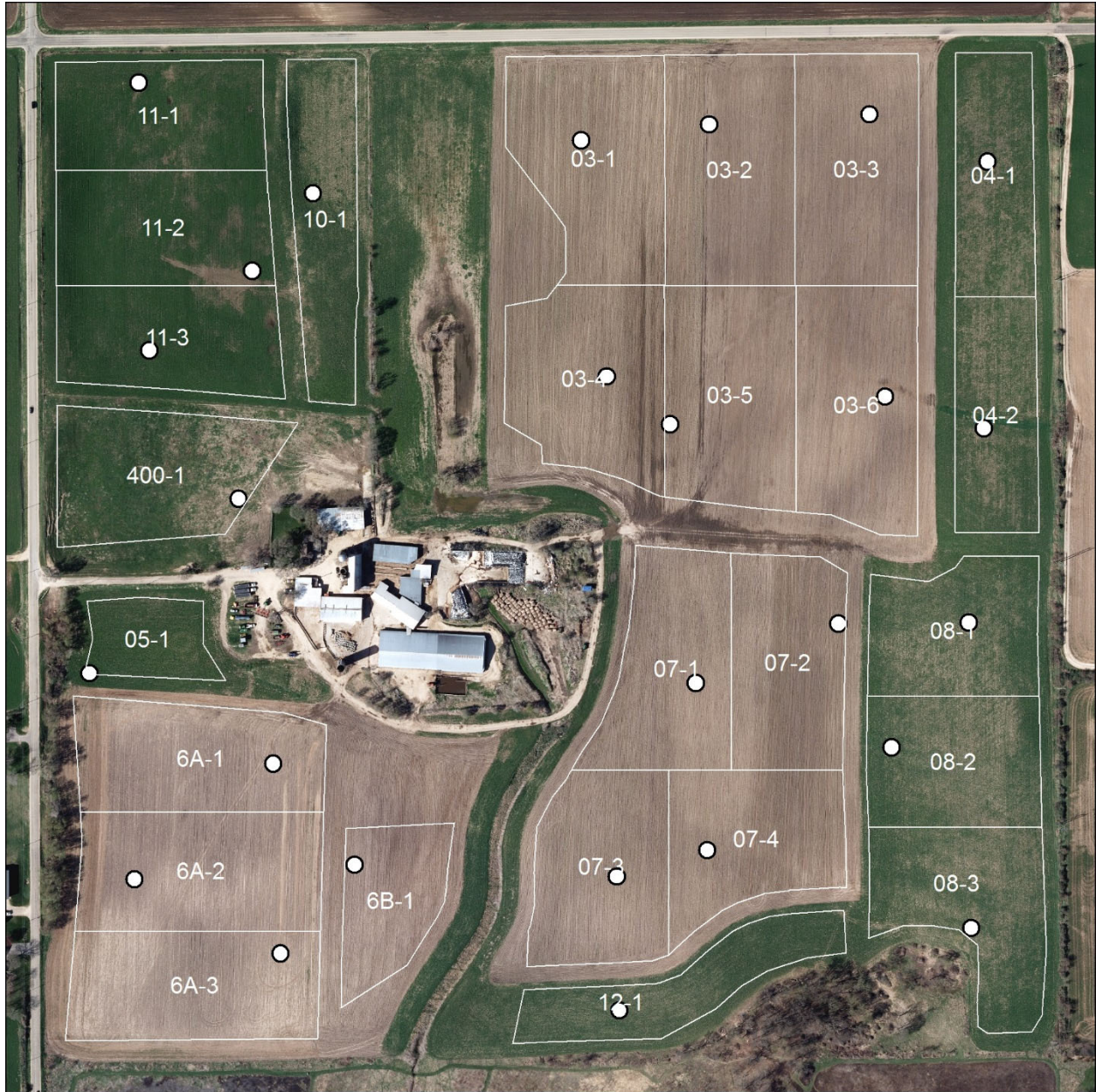
Figure 1. Sample grid and points for the Acker farm. Field boundaries were buffered in by 30 feet to avoid possibly atypical soil conditions. Fields were then trimmed to exclude areas in the permanent pool of the wetland basins. Remaining areas were then divided into approximately equal areas no greater than 5 acres by hand digitizing. Sample points were created in each grid cell with the Create Random Points tool in ArcGIS.
